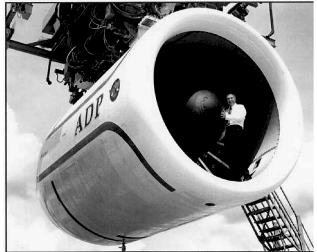
Fig. 60 Advanced ducted propulsor engine (courtesy of P&W).
