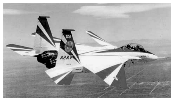
Fig. 48 NASA flight test of pitch/yaw nozzles in F-15 aircraft with P&W F100 engines.
